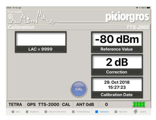
The user can do the calibration in case that they have a calibrated TETRA test set in combination with base station simulator mode (like the Aeroflex IFR3901).
